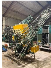
Former Airtec Spray in conversion to convental sprayer. 10/18/20 metre Boom, hydraulic raise/lower tilt, 840 litre tank, clean water tank, stainless steel induction hopper.
