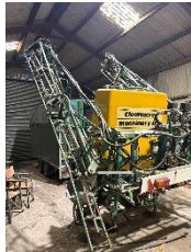
Former Airtec Spray in conversion to convental sprayer. 10/18/20 metre Boom, hydraulic raise/lower tilt, 840 litre tank, clean water tank, stainless steel induction hopper.
