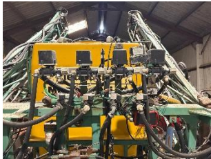
Former Airtec Spray in conversion to convental sprayer. 10/18/20 metre Boom, hydraulic raise/lower tilt, 840 litre tank, clean water tank, stainless steel induction hopper.
